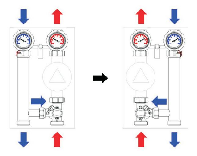
The pump group is pre - assembled for the upper supply type on the right side of the water supply
